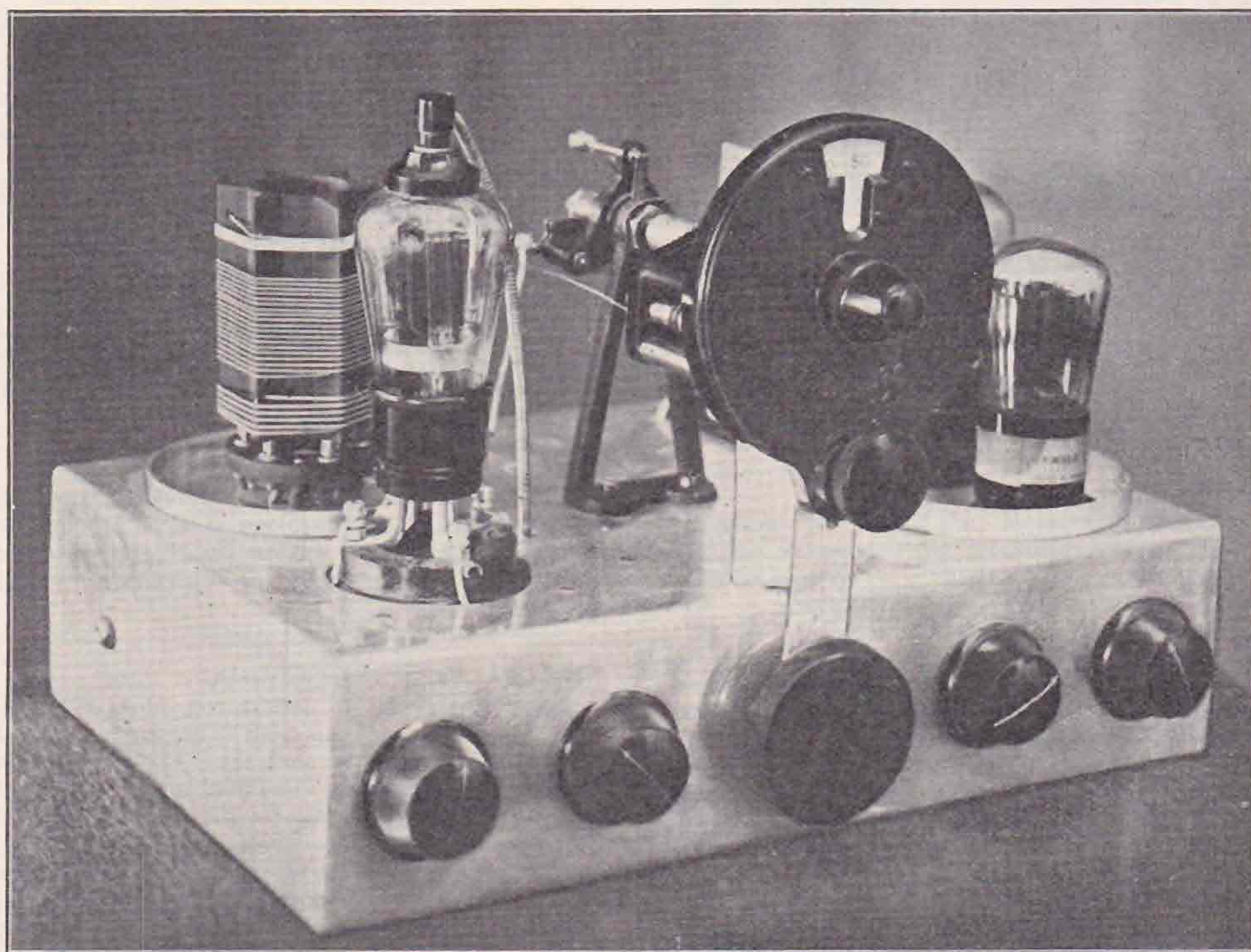
Fig. 2. Front view of Receiver with screening cans removed. Note the method of assembling the tuning condensers.
